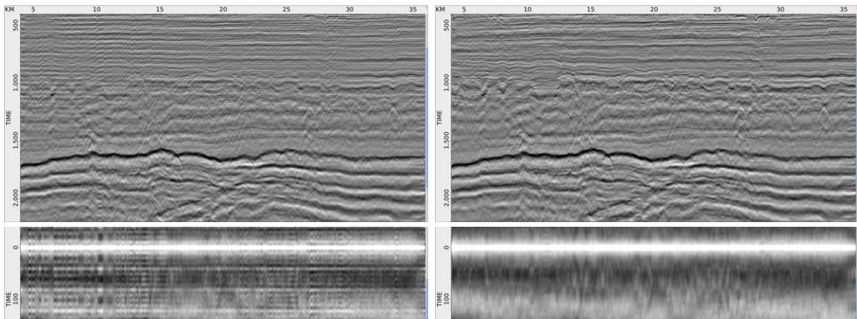
Figure 6: NMO stacks (top) and their autocorrelations (bottom) before demultiple, with deterministic de-ghosting (left) and adaptive de-ghosting (right).
