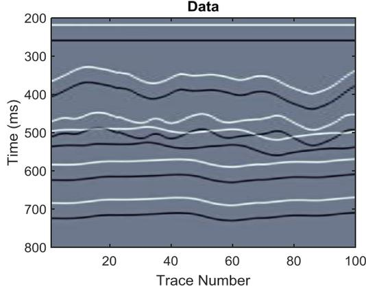
Figure 1: Synthetic data representative of a common- $p$  section, where the delay time between ghost and primary is constant. Primary events appear as white pulses, and the associated black ghosts have a 40msec delay with respect to the primaries.
