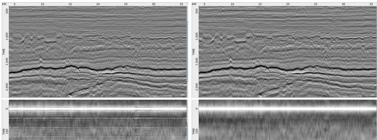
Figure 7 : NMO stacks (top) and their autocorrelations (bottom) after demultiple, with deterministic de-ghosting (left) and adaptive de-ghosting (right).
