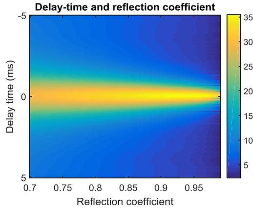
Figure 4: Kurtosis of the joint estimation of delay-time and reflection coefficient.
