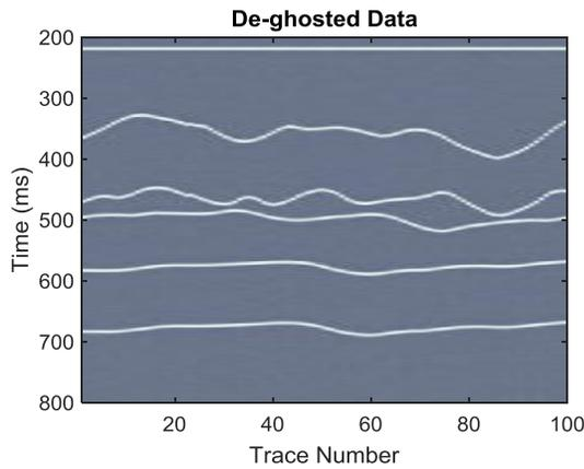
Figure 5: De-ghosting result for the data in Figure 1, after joint optimisation of delay-time and reflection coefficient based on the kurtosis values shown in Figure 4.
